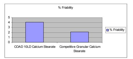
Fines were removed by sieving thru a 140 mesh. 20g of BB's were added to residual on the 140 mesh screen and shaken for 15 minutes. Fines collected. % Friability = (weighed amount collected)(100)/original sample weight.
